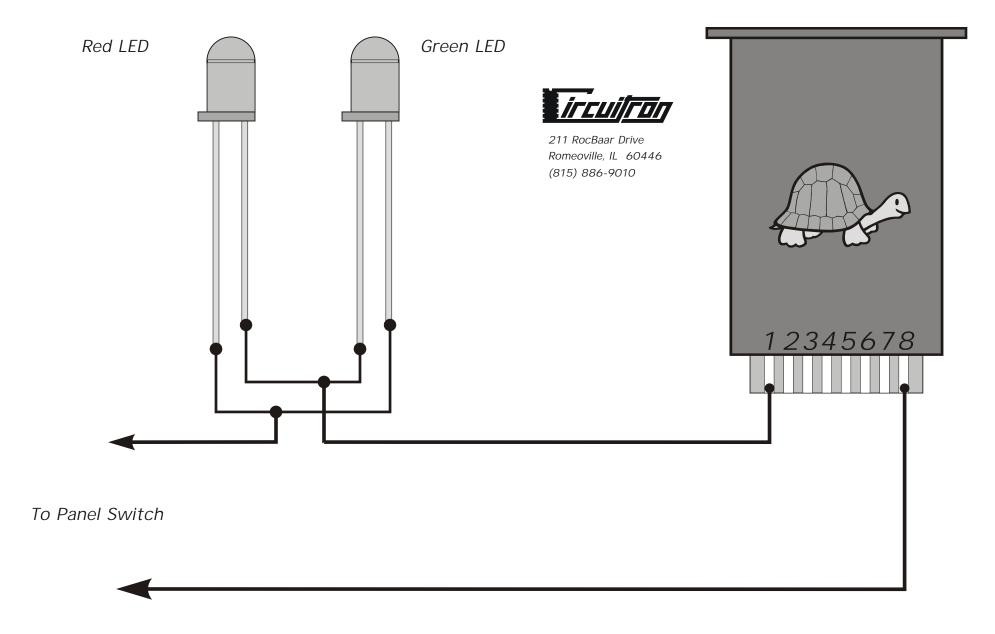
Note: Do not use additional resistors. The resistance of the TORTOISE motor is about 600 ohms, an ideal limiting resistance for LEDs.
